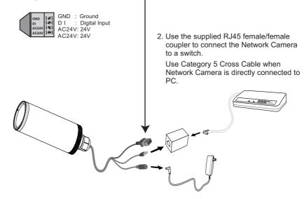
3. Connect the power cable from the Network Camera to a power outlet.
