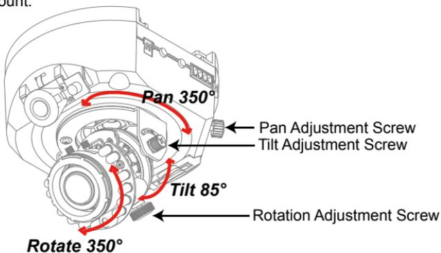
DO NOT over rotate the lens. Doing so will damage the camera lens module
