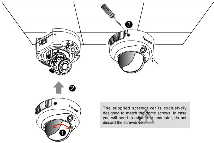
The supplied screwdriver is exclusively designed to match the dome screws. In case you will need to adjust the lens later, do not discard the screwdriver.
