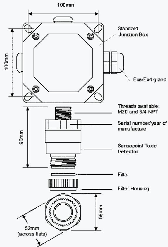
Sensepoint flammable and toxic gas detectors are installed using suitable Exd or Exe junction boxes. The standard junction box available from Honeywell Analytics includes an earth continuity plate for added RFI protection. The detectors have a choice of mounting thread size to match local preferences.
