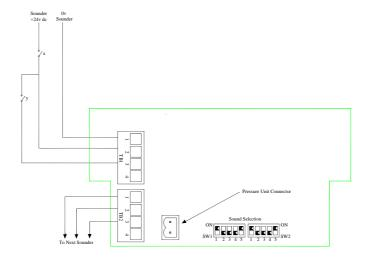
A. Two stage alarm by third core Line monitoring by supply reversal Select alarm stage 1 on SW1 Select alarm stage 2 on SW2
