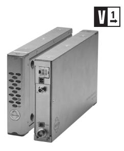
The **FT8301A/FR8301A** fiber transmitter and receiver provide the ability to transmit one composite video channel over one optical fiber. The **FT8301A** transmitter and the **FR8301A** receiver are available in multimode and single-mode versions. When using single-mode fiber, the **FT8301A** transmitter and the **FR8301A** receiver offer an exceptional optical power budget of 28 dB and provide a transmission distance of up to 46 km.
