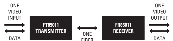
SINGLE-CHANNEL VIDEO AND BIDIRECTIONAL DATA APPLICATION
