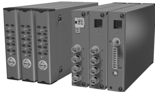
The **FT85081/FR85081** fiber transmitter and receiver provide the ability to transmit up to eight unidirectional composite video channels and one bidirectional data channel over one optical fiber. The **FT85081** transmitter and the **FR85081** receiver are available in multimode and single-mode versions.
