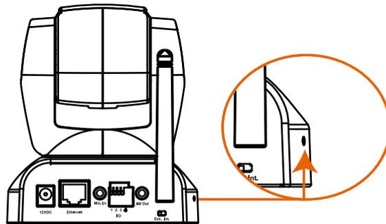
The reset button is used to reset the system or restore the factory default settings. Sometimes resetting the system can return the camera to normal operation. If the system problems remain after rebooting, restore the factory settings and install again.
