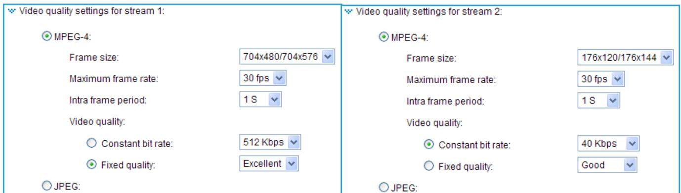
There are four parameters provided in MPEG-4 mode which allow you to adjust the video performance:
