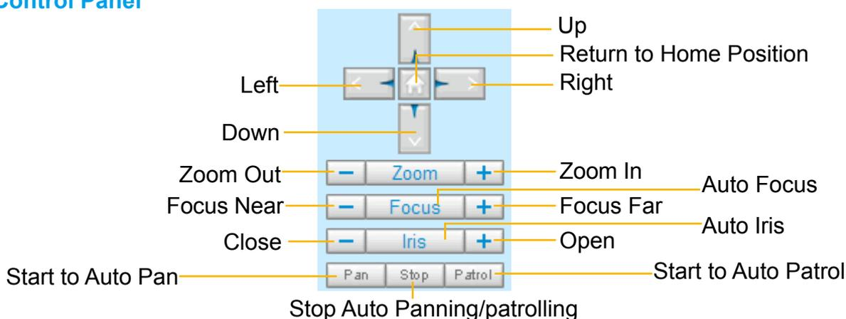
**Pan:** Click this button to start the auto pan. When the current position is Home or on the left side of Home, the camera starts panning from the current position to the left-most position, then to the right-most position, and finally backward to the original position. When the current position is on the right side of Home, the camera starts panning from the current position to the right-most position, then to the left-most position, and finally backward to the original position.
