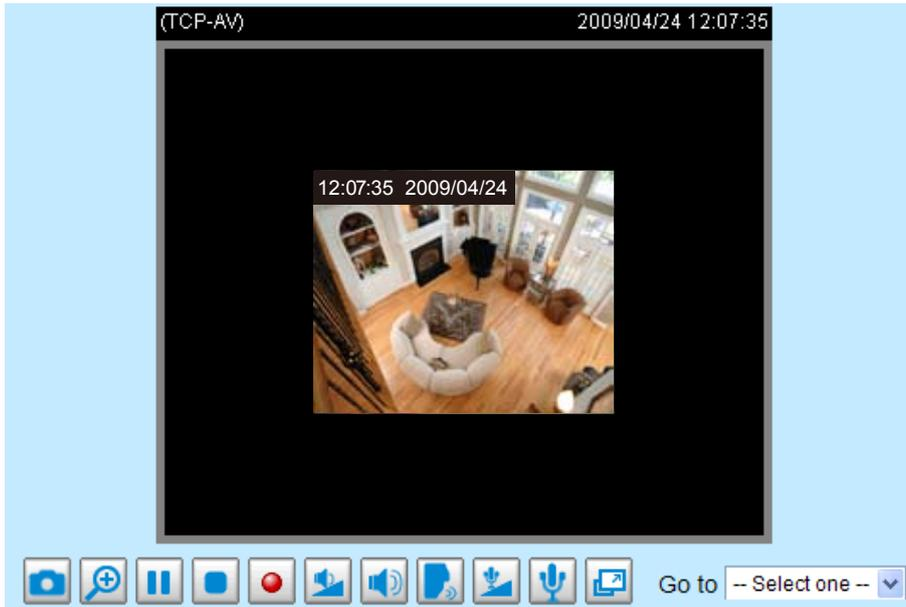
Enable time shift caching stream **Advanced Mode**: Check this item to enable the time shift cache stream on the Network Camera, which will store video in the camera's embedded memory for a period of time depending on the cache memory of each Network Camera. This function can work seamlessly with VIVOTEK's ST7501 recording software. When an event occurs, the recording software can request time shift cache stream from the camera, which allows the user to get an earlier video data.
