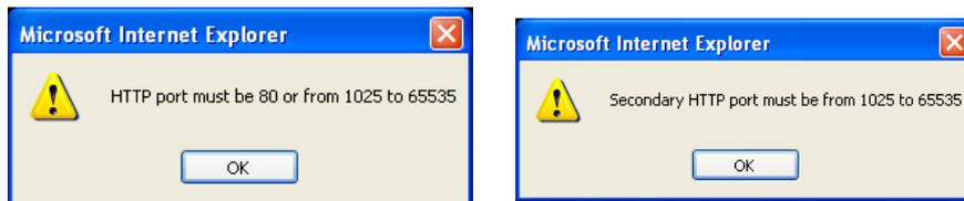
To access the Network Camera on the LAN, both the HTTP port and secondary HTTP port can be used to access the Network Camera. For example, when the HTTP port is set to 80 and the secondary HTTP port is set to 8080, refer to the list below for the Network Camera's IP address.
