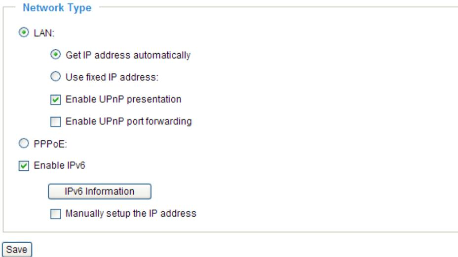
When IPv6 is enabled, by default, the network camera will listen to router advertisements and be assigned with a link-local IPv6 address accordingly.
