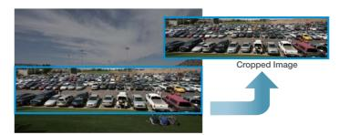
The IP8161 provides electronic pan/tilt/zoom functions, allowing users to move to a target region in the full view window without changing the camera direction physically. Since only the target region will be transmitted for individual viewing, bandwidth requirements are significantly reduced.
